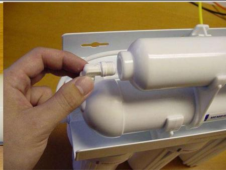
\*if you have quick connect fitting, push plastic ring against fitting, pull out tubing
