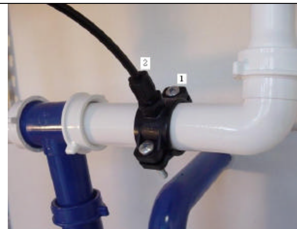
put the complementary piece and clamp them together with the two bolts. (1) Tighten the two bolts evenly. (2) Connect tubing
