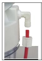
**NOTE:** The system uses compression fitting connections: When connecting tubing to the system, first, you must unscrew the compression nut off the fitting, then pass the tubing through the compression nut about 1", then screw on to the fitting, then use a 5/8" wrench to tighten the nut until the thread is not visible. Don't over-tighten it.
