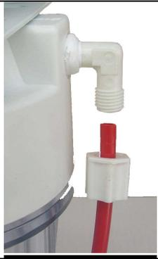
**NOTE: The system uses compression fitting connections:** When connecting tubing to the system, first, you must unscrew the compression nut off the fitting, then pass the tubing through the compression nut about 1", then screw on to the fitting, then use a 5/8" wrench to tighten the nut until the thread is not visible. Don't over-tighten it.
